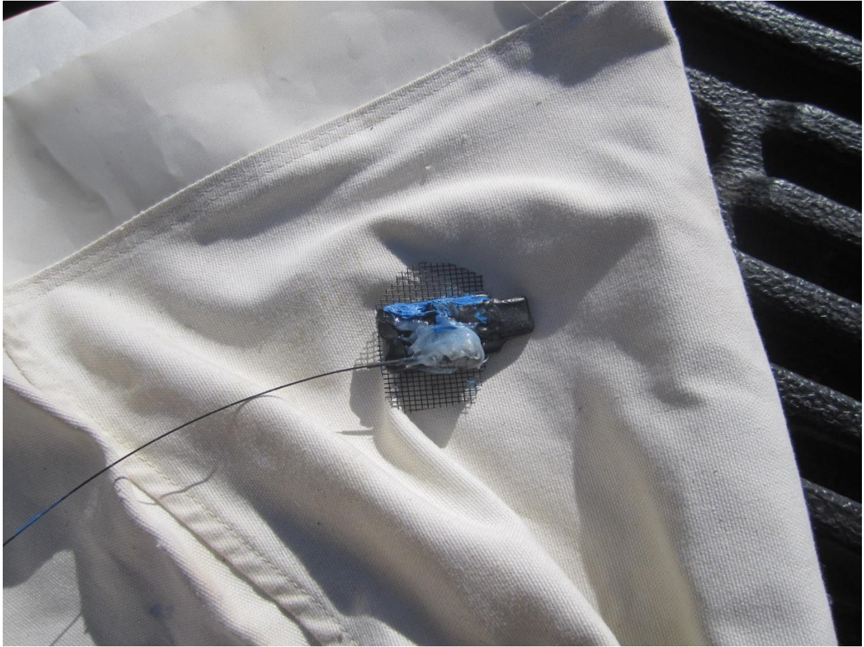
GPS unit with the 1.9 gram transmitter glued to the GPS.
