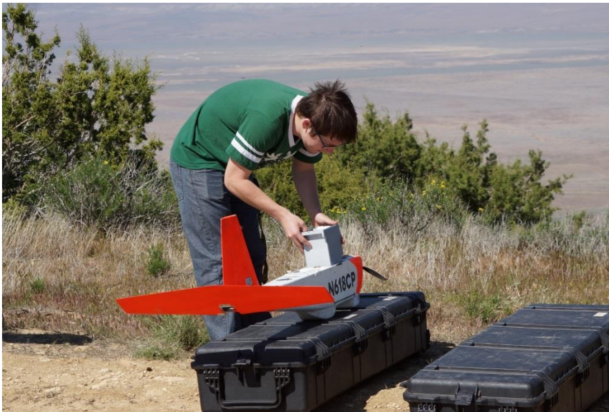
Figure 8. Inserting base station/receiver payload module into RQ-20.
